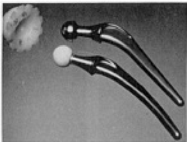
Fig. 10 Charnley low-friction hip joint prosthesis equipped with a polymeric UHMWPE acetabular cup and either a stainless steel (top) or an Al 2 O 3 ceramic (bottom) femoral head
