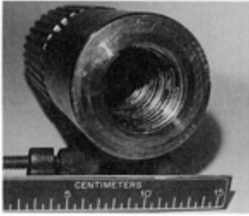
Fig. 3 Valve stem nut showing wear of threads
