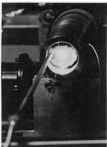
Fig. 15 Laser cladding of small-bore pipes. Source: Ref 46
