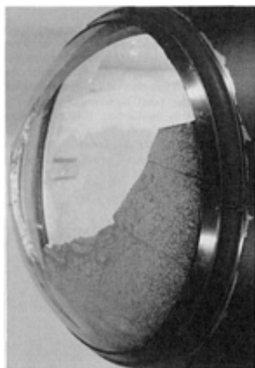
Fig. 2 Rain erosion effects on a Maverick missile dome made of coated zinc sulfide that was exposed for 10 s at a speed of about 210 m/s (690 ft/s). The dome itself suffered catastrophic damage, and erosion is also seen on the filled elastomeric mounting ring. Courtesy of G.F. Schmitt, Jr., Materials Laboratory, Wright Research and Development Center, Department of the Air Force
